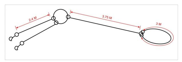
**Remark:** Please note that this diagram is informative only and used for a standard boat with standard measurements – always check the advise given above – weight and length are decisive for triangle measurements.
