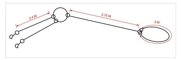
**<u>Remark:</u>** Please note that this diagram is informative only and used for a standard boat with standard measurements – always check the advice given above – weight and length are decisive for triangle measurement
